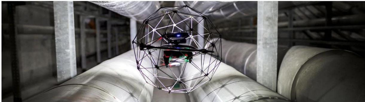
**Fig. 9.** Elios drone. Source: <https://www.flyability.com/>
