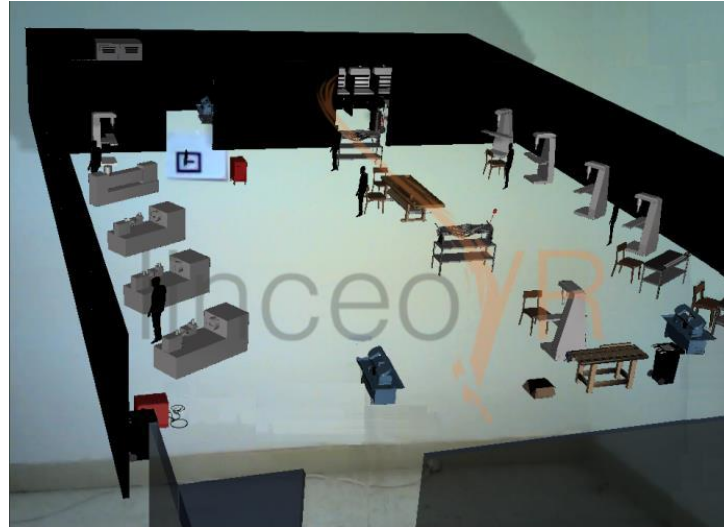
Figure 12: Augmented Reality used for factory planning [15]
