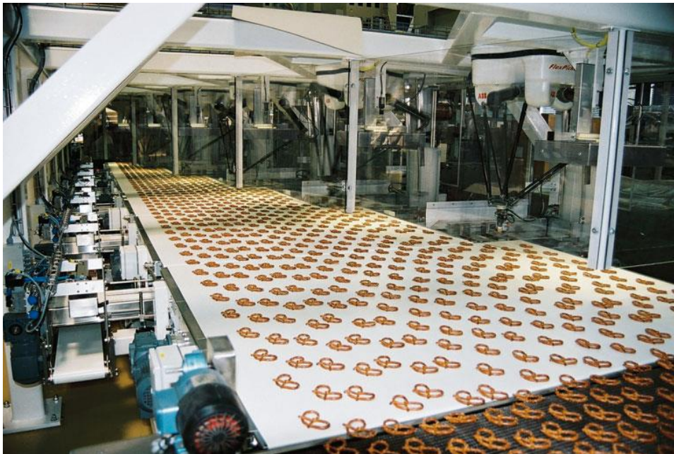
Figure 1. Robots picking pretzels from a conveyor belt.(Source ABB)
