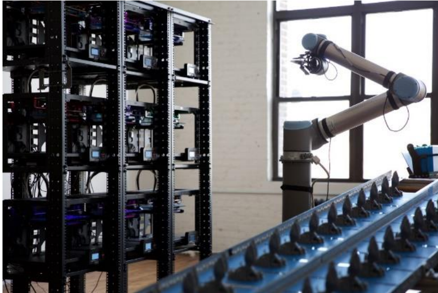
Figure 9. 3DP process automation (Image credits: Voodoo Manufacturing)
