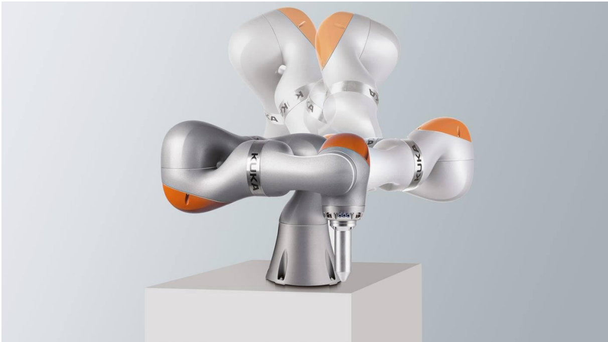
Figure 5 LBR iiwa by Kuka – world's first sensitive robot approved for Human-Robot collaborative work. Photo: Kuka
